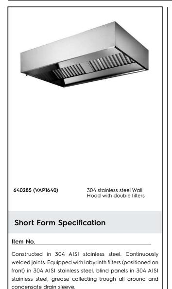
The rear baffle directs the fumes towards the filter surface, condensing the steam which is then conveyed through the outer ducting into the discharge. Suitable for use where large volumes of steam must be exhausted (i.e. ovens, dishwashers, pan washers, etc.)
