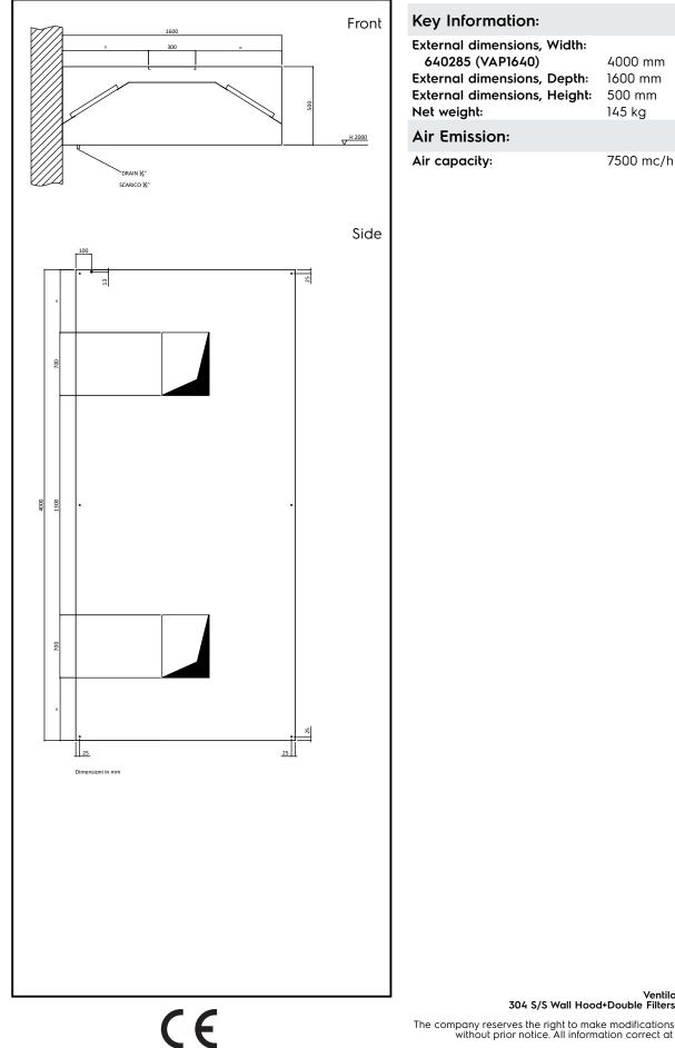
Ventilation Equipment 304 S/S Wall Hood+Double Filters 4000X1600mm
